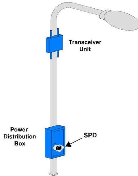
Figure 4. Example of small cell installation.
