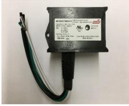
The MPD Series is a modular surge protective device (SPD), featuring an IP65 enclosure rating and available with operating voltages of: 120VAC, 277VAC, 347VAC and 480VAC. MPD Series is UL 1449 – Type 4CA recognized and can be connected in series and parallel with the load.
