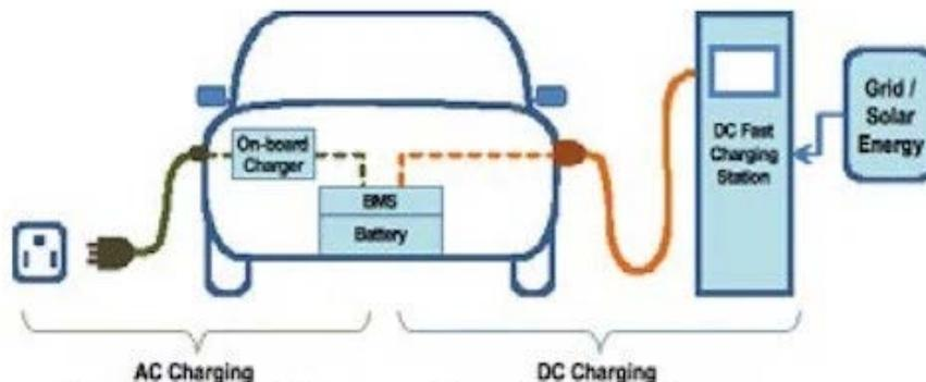
Figure 1 <sup>(4)</sup>. AC charging vs DC charging
