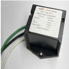
The MPDS Series is a smaller form factor of our MPD Series, featuring an IP65 enclosure rating. The MPDS Series utilizes metal oxide varistors to provide a protection package for use in many applications. A metal oxide varistor will divert, absorb and dissipate the energy of a transient. MPDS Series is UL 1449 – Type 4CA/Type5 recognized and can be connected in series and parallel. The MPDS Series is available with operating voltages of: 120VAC, 277VAC, 347VAC, and 480VAC.
